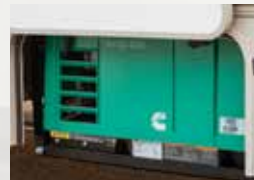
Standard ONAN 4.0kw gas generator with auto transfer switch.
