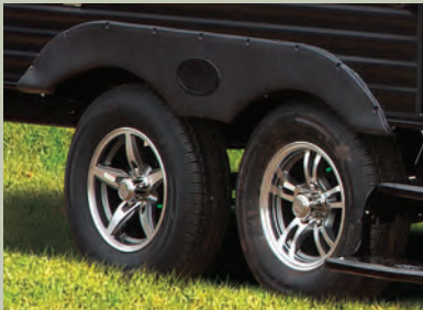
Tandem axles enhance stability
