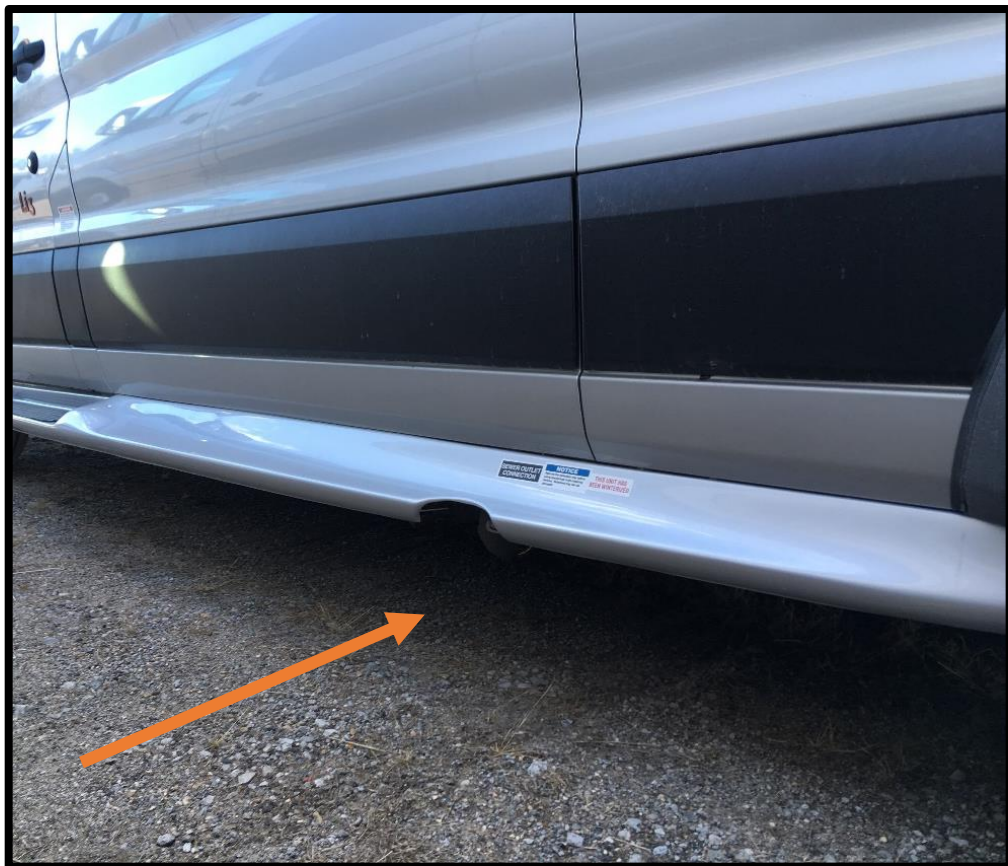
NEW! DRIVER SIDE RUNNING BOARD NOTCH ALLOWS EASIER ACCESS TO THE TERMINATION VALVE
