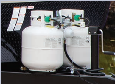
Double 20 lb. LP tanks
