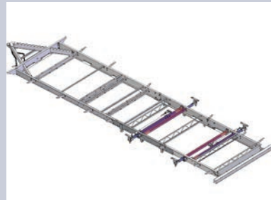
Norco NXG chassis featuring E-Coat technology
