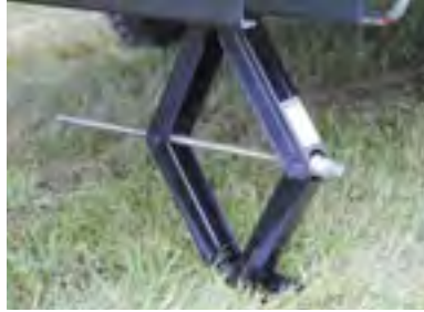
The four heavy duty scissor-style stabilizing jacks extend and retract easily using your cordless drill and the provided drill bit.
