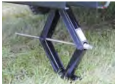
The four heavy duty scissor-style stabilizing jacks extend and retract easily using your cordless drill and provided drill bit.
