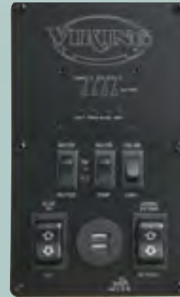
Interior Command Center controls awning, interior lighting, slide out, water heater/pump, battery indicator lights, and has two USB outlets.
