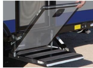
The E-Z Swing Stepper Door with hydraulic assist, operates in seconds and provides the largest, most stable step platform in the industry.
