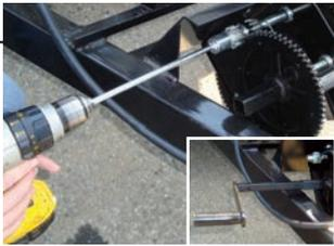
Easy-to-use dual drive winch and drill socket, with your cordless drill, raises or lowers the roof in under 30 seconds. A manual crank is also provided.
