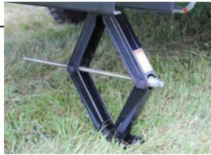
The four heavy duty scissor-style stabilizing jacks extend and retract easily using your cordless drill and the provided drill socket.
