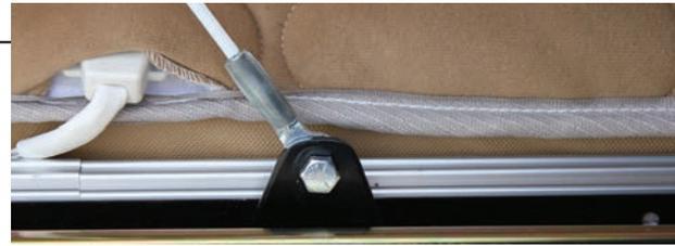
This exclusive "Glide-N-Lock" cable supported bed system eliminates the need for support poles under the beds. Simply pull out the bed, click and it's locked into place.
