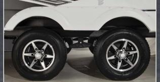
Stable-Ryd<sup>®</sup> Spread Axles provide better weight distribution, handling and improved towing.
