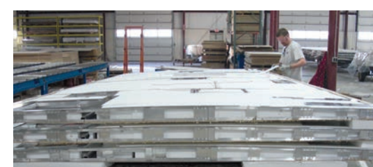
Aluminum Reinforced Vacuum-bonded Roof
