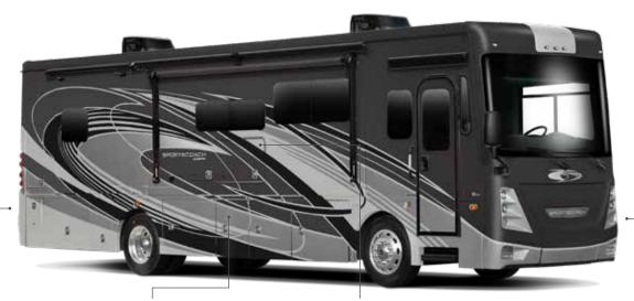
With a 360HP ISB Cummins rear diesel engine and a 6-speed Allison 3,000 MH automatic transmission, Sportscoach gets 800 lbs./ft. of torque and has a 10,000 pound towing capacity.
