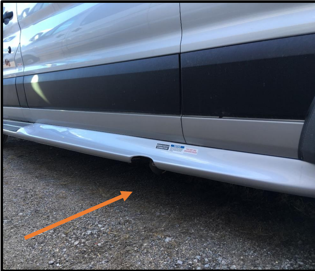
DRIVER SIDE RUNNING BOARD NOTCH ALLOWS EASIER ACCESS TO THE TERMINATION VALVE
