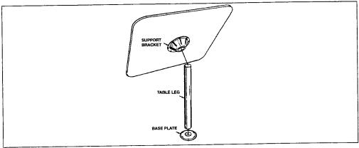
(To assemble, insert table leg into base plate. Lower table support bracket onto the leg.)
