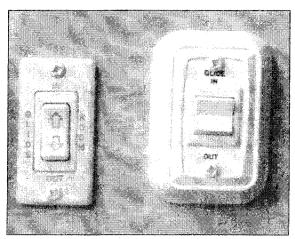
**IMPORTANT:** Holding the switch after the room has reached the full extent of travel, either in or out, could result in damage to the mechanism or the structure of the trailer.
