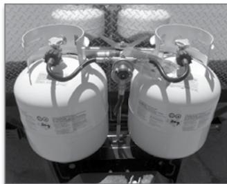
also allows expansion space for the liquid. If the tank were completely full, a rise in outside temperature could result in relief valve discharge of LP gas.
