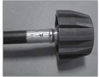
The average life of an LP hose is approximately 2 to 3 years. Inspect the hose before each camping season, and when having the tank filled. Look for signs of deterioration such as cracks or loss of flexibility. Protect the hose from the direct rays of the sun, if possible, to help slow down the aging process. When the hose is replaced, always replace it with a hose of the same type and rating (check with your dealer).
