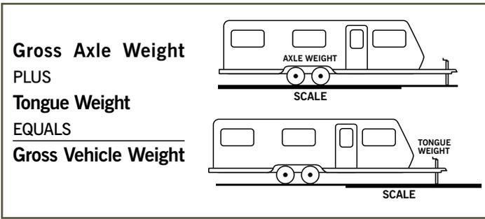
**NOTE:** Gross axle weight is determined with all tires on the scale. Side to side weight distribution is determined by weighing each side independently.
