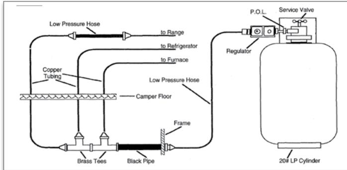
Road vibration can loosen LP gas fittings and connections. It is important to check your LP system for leaks at least every 5,000 towing miles, and whenever the tank is filled.
